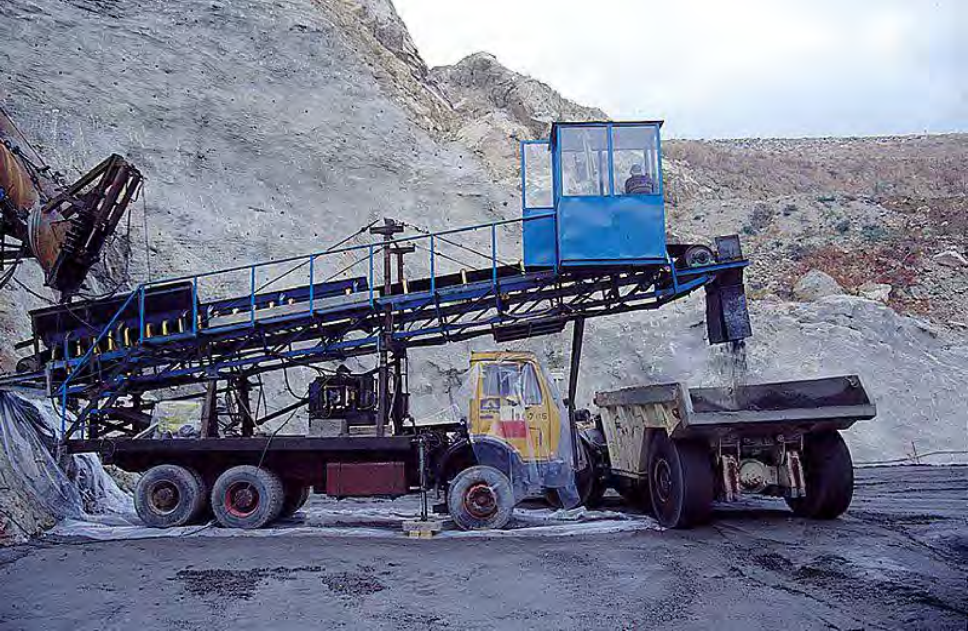
•Truck mounted belt conveyor, end sluice gate.
