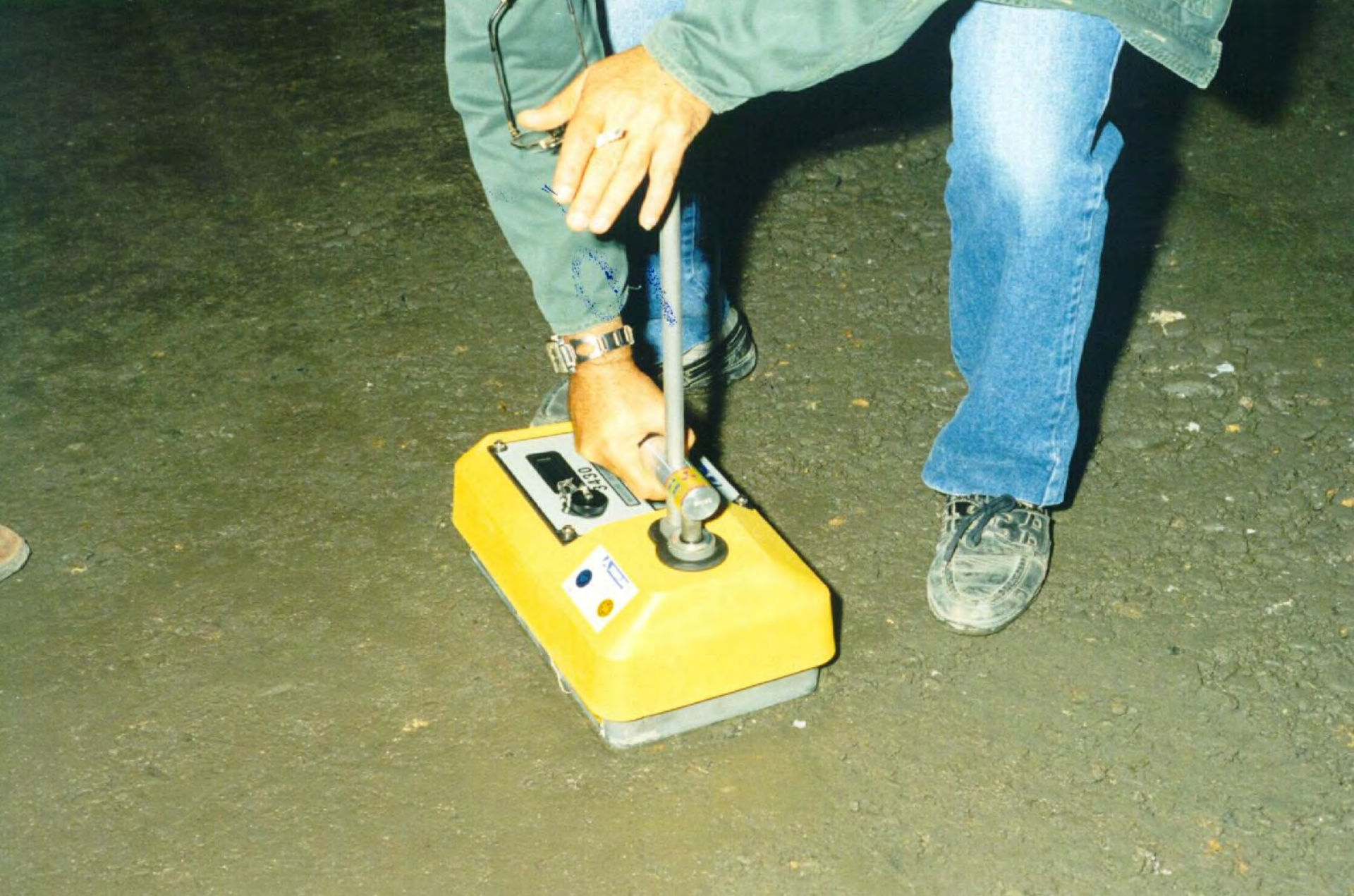
RCC testing (nuclear densiometer).
