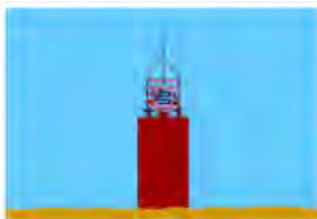
Caisson touchdown & penetrates initially by own weight
