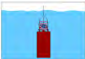
Lower caisson + suction pump
