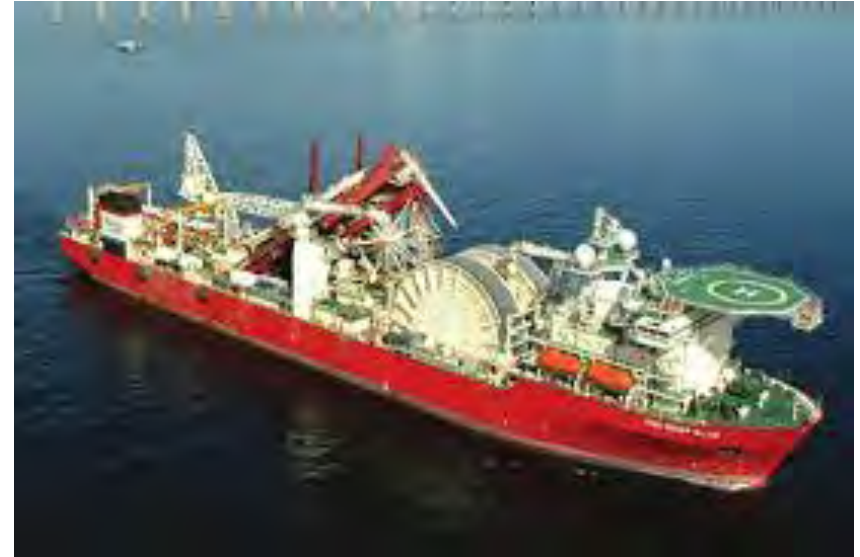
REELING PIPELAY SHIP
